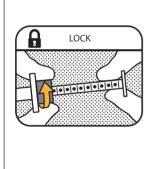
right hand and lock the ringstop by turning it away from you. Confirm that the ring-stop is in the locked position on the dosing syringe by making sure it is not freely moveable.
