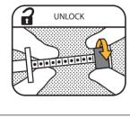
hand and unlock the green ringstop by turning it towards you until it is able to slide freely.
